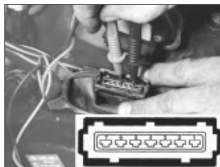
10.2a Check for voltage at terminals 2 and 4 on the control unit electrical connector (Bosch system shown)
