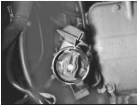
8.7 Mark the relationship of the rotor to the distributor housing (arrowed)
